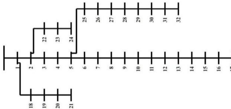
**Figure 2.** 33-bus test system
