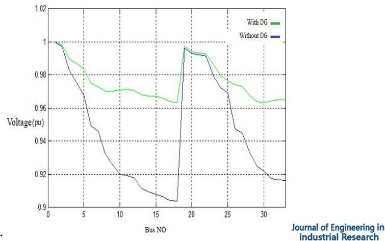
**Figure 5.** Voltage profile after installing the multiple distributed generators in the constant power load
