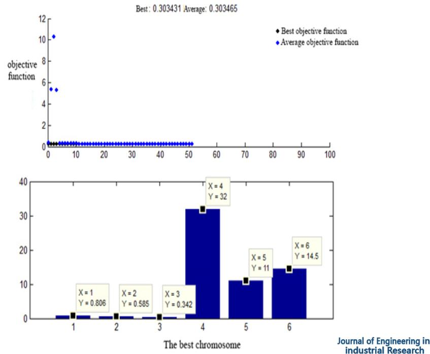
**Figure 4.** The best location for installation, calculated by the genetic algorithm in the constant power load
