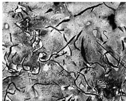
Figure 3: Whitening of cast iron due to the penetration of tellurium.
