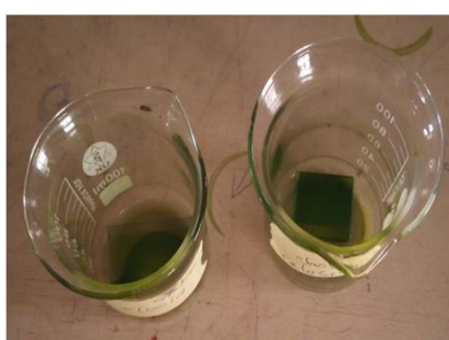
Figure 2: The photoanode deposition on the FTO glass. Figure 3: The dye-coated photoanode layers.
