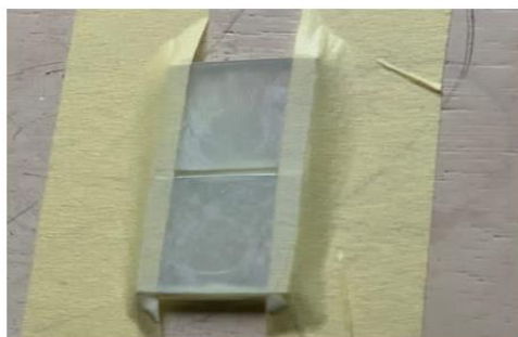
Figure 2: The photoanode deposition on the FTO glass. Figure 3: The dye-coated photoanode layers.
