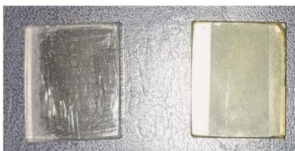
Figure 4: The conductive side of the counter electrode coated with a pencil carbon.
