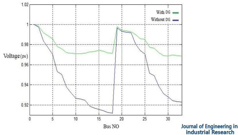
Figure 6. The voltage profile after installing the multiple distributed generators in the constant current load
