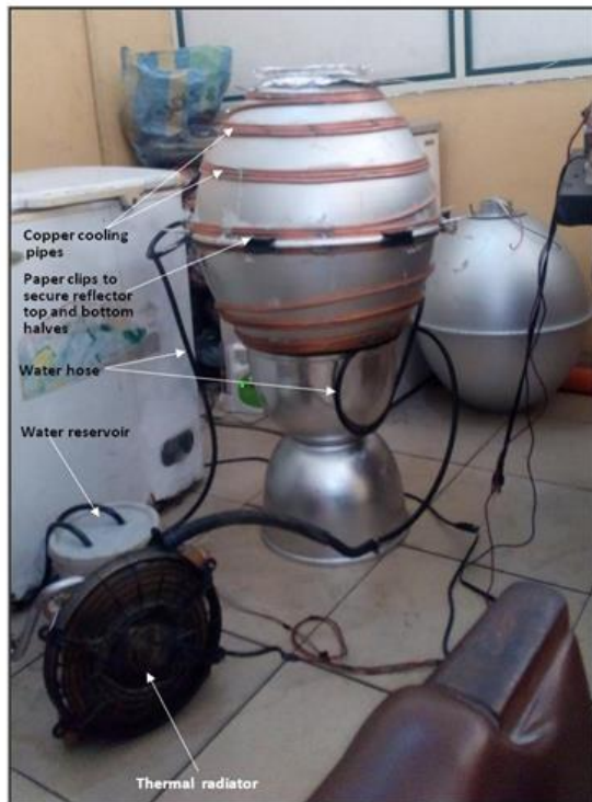
Figure 5: The assembled furnace and the cooling accessories.
