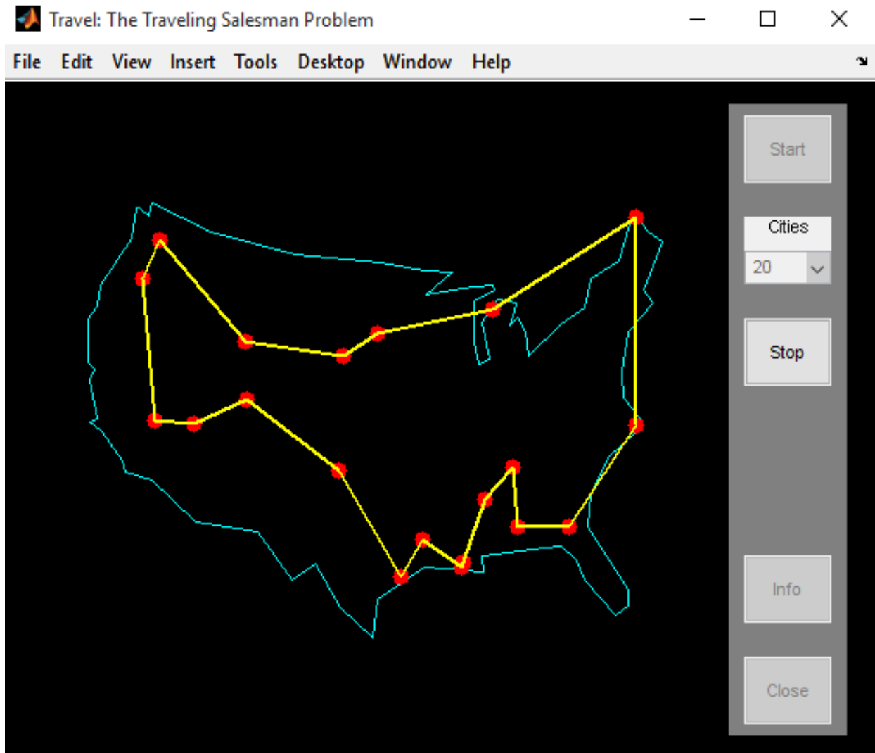
Figure 2. Location/Cities Spanning for TSP solver during execution in MATLAB
